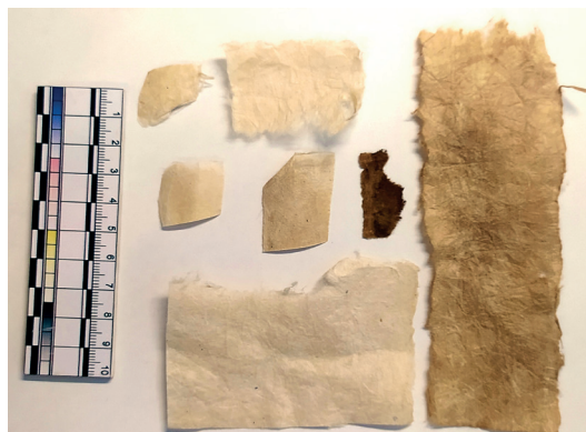
Fig. 5. Preparation of a new base for the duplication procedure. Far right - modern Samarkand paper specially processed by us for duplication. Next to it (on the left) - one of the fragments of paper found in the Ili-Balyk burial ground. Other samples of modern Samarkand paper at different stages of preparation as a base for duplication
